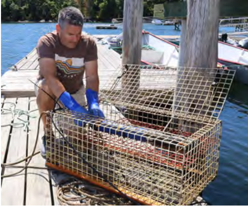
Photo 1: Friends of Casco Bay deploys its sondes using a modified lobster trap.
