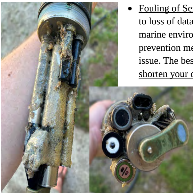
Photo 2: Tunicates and algae have collected on this data sonde. While the sonde’s wiper has kept sensors relatively clean, the best way to reduce biofouling is to shorten deployment time
