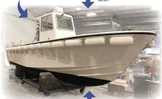
Modified "V" hull especially designed to carry 650 gallons of sewage — more than twice our current capacity.
